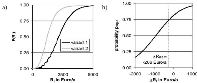
Fig. 4. Comparison of reimbursements for variants with improvement of the telecontrol (reducing switching duration from 1h to 0.5h),  $l_{line}=0.65$  km, tariff01,  $T_{obs} = 20a$ ,  $R_i$  acc. to eq. (3).
