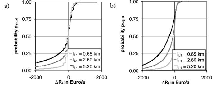
Fig. 10. Significance probability  $p_{sig d}$  for conversion of radial to open loop structure, different line lengths  $l_{L1}= l_{L2}$ , tariff01
