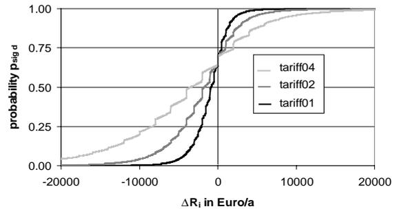
Fig. 6. Significance probability  $p_{sig,d}$  for variants with improvement of the telecontrol (reducing switching duration from 1h to 0.5h),  $l_{line}=0.65$  km,  $T_{obs} = 5a$ , different reimbursement factors  $r_E$
