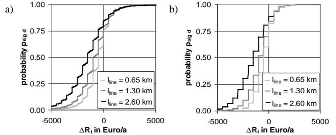
Fig. 8. Significance probability  $p_{sig_d}$  for variants with improvement of the protection system, different line lengths  $l_{line}$ ,  $T_{obs}=5a$
