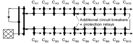
Fig. 7. Test-system II with upgraded protection system
