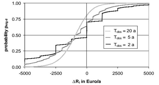
Fig. 5. Significance probability  $p_{sig,d}$  for variants with improvement of the telecontrol (reducing switching duration from 1h to 0.5h),  $l_{line}=0.65$  km, tariff01, different observation periods  $T_{obs}$ .
