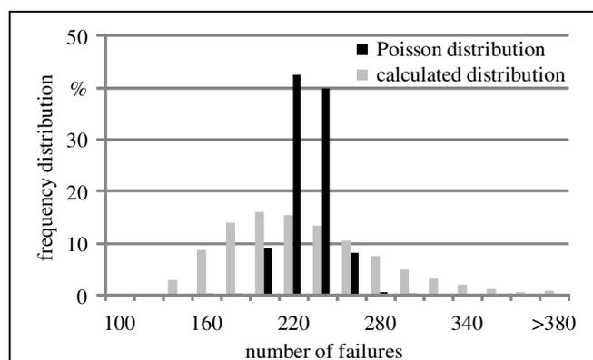
**Figure 5: Distribution of the simulated number of failures in comparison to the Poisson distribution**
