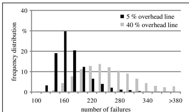
**Figure 6: Distribution of the simulated number of failures for different overhead line rates**
