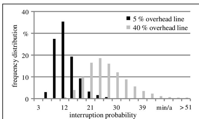
**Figure 7: Distribution of the interruption probability for different overhead line rates**
