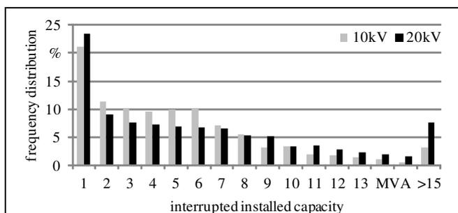
**Figure 3: Distribution for the interruption extent of an overhead line at different voltage levels**
