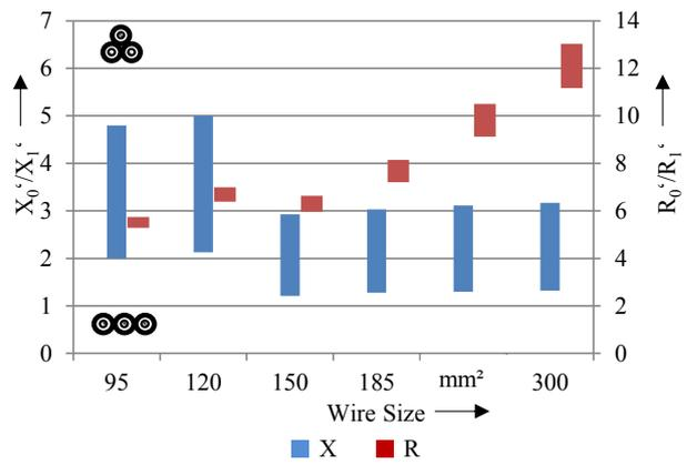
**Figure 8** Range of possible  $R_0'/R_1'$  and  $X_0'/X_1'$  ratios of different wire sizes, exemplary for N2XSY Cable [8]
