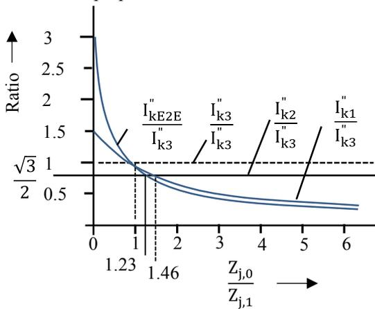
**Figure 7** Influence of  $Z_0/Z_1$ -ratio on short circuit current level at fault location [9]
