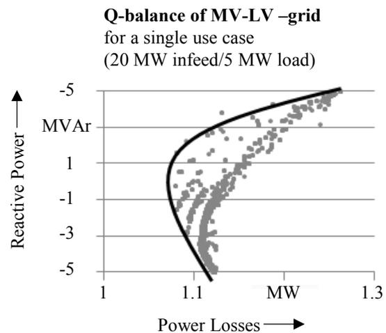
**Figure 6** Power losses against Q-Balance for a single use case
