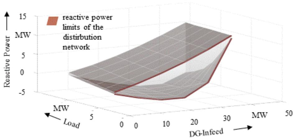
**Figure 5** Reactive power limits of an exemplary rural distribution network
