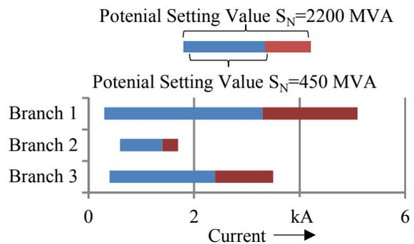
**Figure 9** Exemplary potential setting value in three MV branches dependence on overlay network short-circuit power
