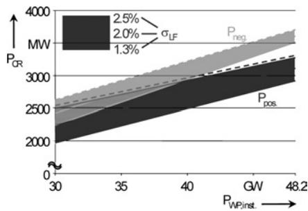
**Figure 7** Demand of control reserve in case of joint control area in Germany
