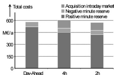
**Figure 5** Total costs for provision of control reserve for an exemplary control area and a total German wind power capacity of 30 GW
