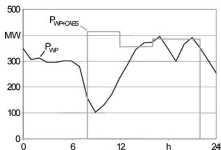
**Figure 8** Concept of refining wind power
