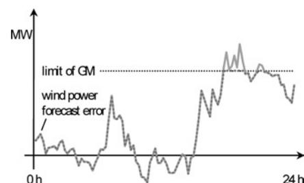
**Figure 1** Wind forecast error before GM and the resulting deviation, which has to be compensated by control reserve
