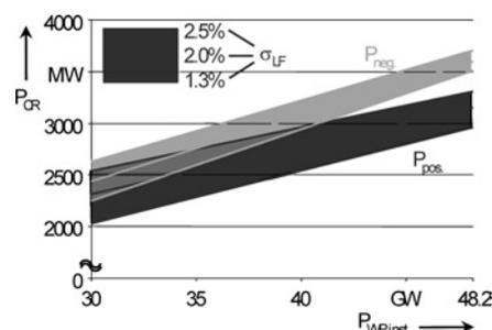
**Figure 6** Demand of control reserve in case of immediate equalisation of wind and load forecast errors between control areas
