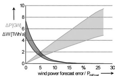
**Figure 2** Demand of control reserve because of wind forecast error and discarded wind power feed-in in dependency on the opted maximum positive wind forecast error
